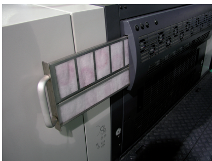
The filter mat is easy to exchange even when the press is running.
