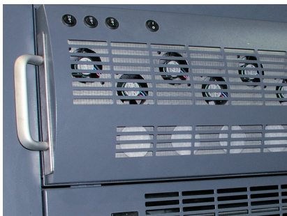
Inking unit guard with inking roller blowing device and integrated ink mist extraction.
