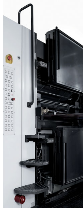
ROTOMAN printing unit with APL™ cassette for fully-automated plate change.
