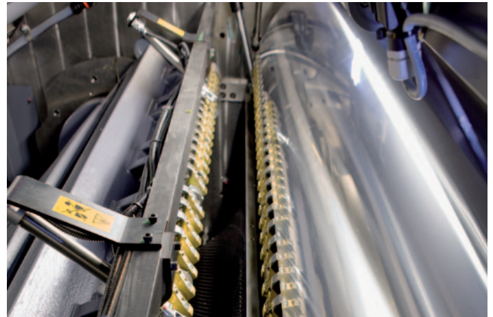
Plates can be changed automatically on the XXL format ROLAND 900 with APL (AutomaticPlateLoading).
