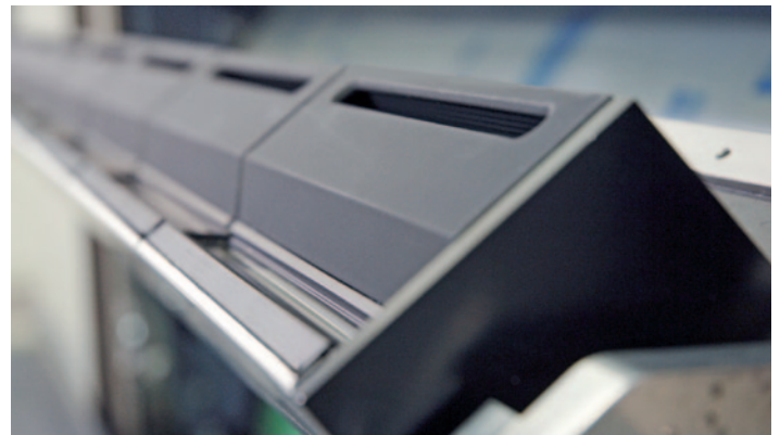
Quality assurance in printing: the ink density measuring and controlling system ROLAND InlineColorPilot.
